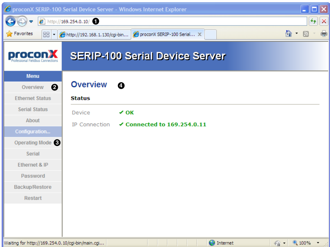
Figure 5.1: Device management and configuration via the web browser
