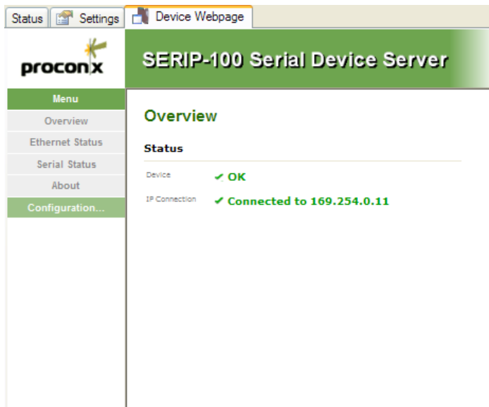
Figure 6.5: SERIP COM Manager device web page pane
