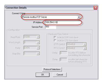
Configure the *ModScan32* data form to point to the *GCP-30 remote control data table 4:0001* as shown below:
