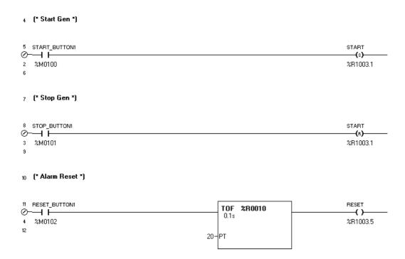
Three buttons on a touch screen implement genset start, stop and alarm reset functions. The start button sets the remote start bit, the stop button resets the remote stop bit. The alarm reset button triggers a run-on timer which keeps output coil %R1003.5 asserted for 2 seconds and then resets this command bit. This makes sure that sure that the command bit is automatically reset and a raising edge generated.
