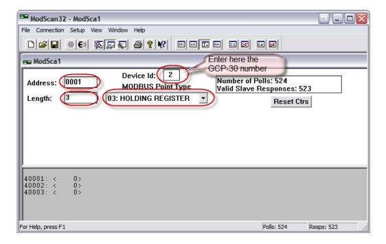
The control word at Modbus address 3 can be set to one of the following decimal values:
