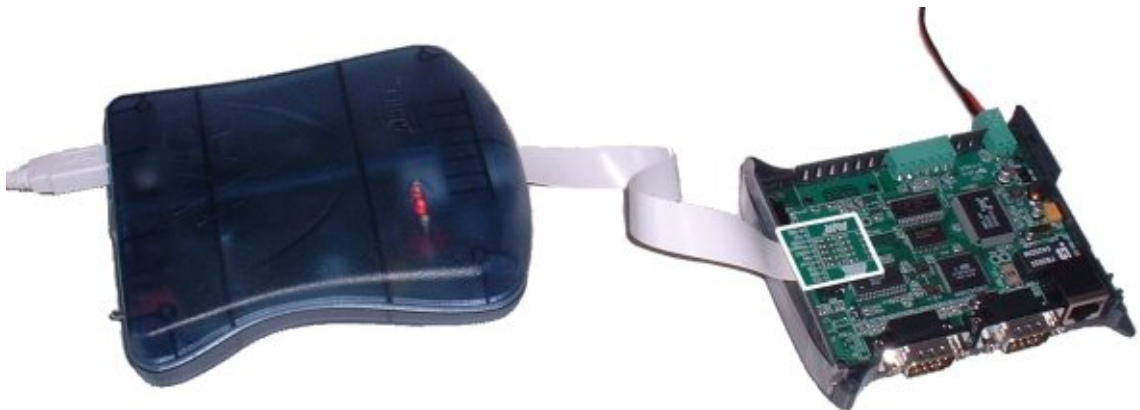
Figure 5.1: JTAGICE mkII connected to XNUT-100 circuit board
