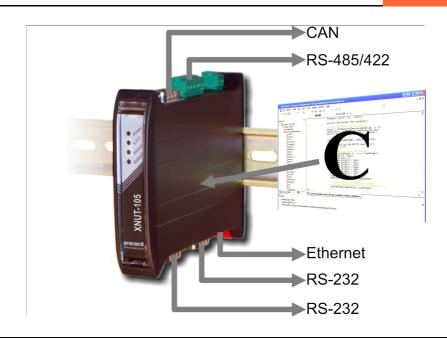
**XNUT-105**, the Ethernet DIN rail Single Board Computer with special features for **Networking** and **Communication** tasks enables you to develop your own IP based control and protocol conversion application based on Nut/OS within a few hours.
